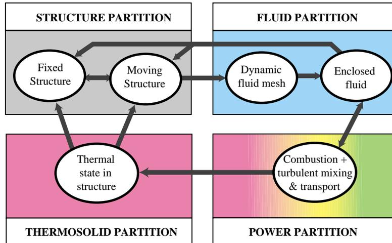
Figure 17. Simulation of a high-temperature gas turbine engine as four-field coupled system.
