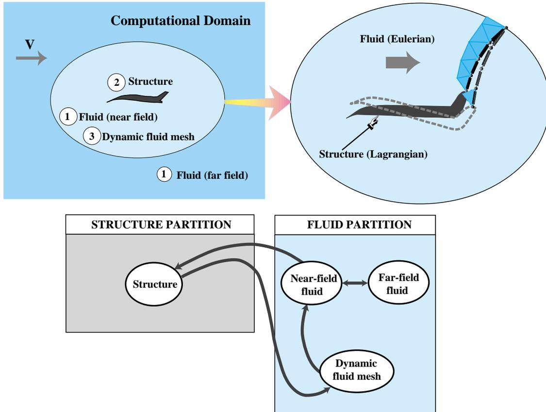
Figure 13. The exterior aeroelastic problem as a three-field, two partition system.
