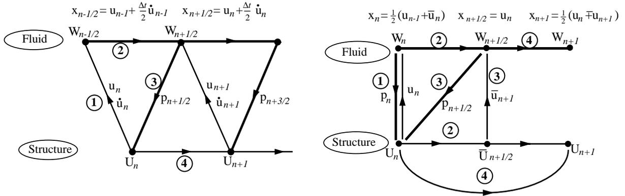
Figure 20. Improved serial and parallel staggered procedure for the exterior aeroelasticity problem.  $U$  and  $W$  are the structure and fluid state variables, respectively. From Ref. [39].
