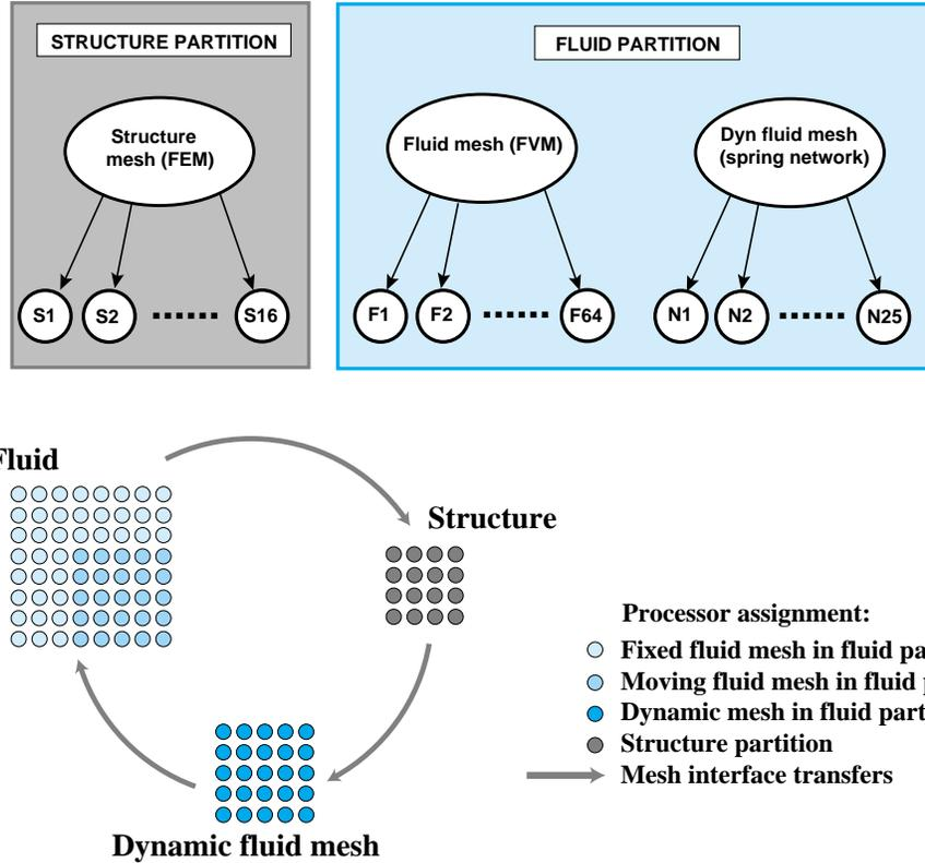
Figure 18. The top figure shows two decomposition levels in parallel analysis of a coupled system: partitions and subdomains; illustrated for the exterior aeroelastic problem. Bottom figure depicts a one-to-one mapping of subdomains to processors of massively parallel computer. A three field partition is shown for illustrative purposes only: in present implementations the dynamic mesh is part of the fluid solver.
