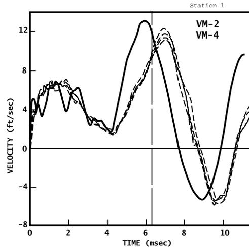
Figure 21. Computed (solid line) and Measured (dashed lines) Longitudinal Velocity Responses to End-On Attack
