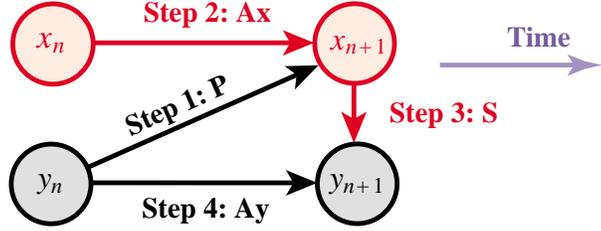
Figure 6. Interfield+intrafield time-stepping diagram of the staggered solution steps listed in Figure 3.
