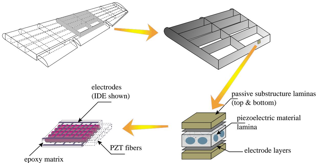
Figure 15. Piezoelectric control of wing shape for vibration and flutter suppression
