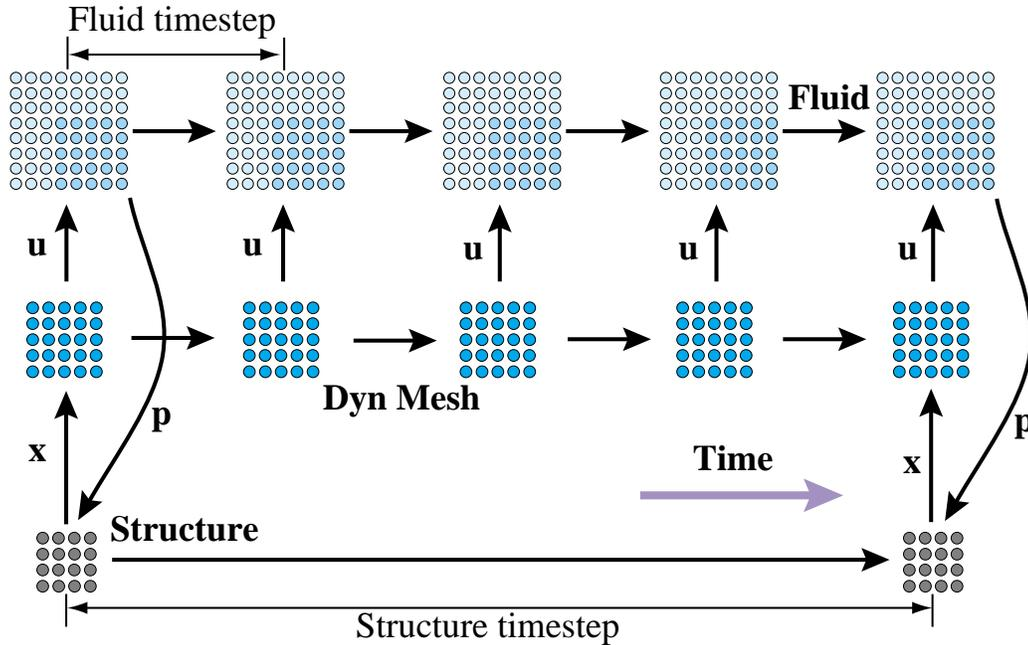
Figure 19. Parallel time stepping of the mapping of Figure 18. This is an idealized diagram prepared in 1993. Adaptation to new architectures and algorithm development have produced variations outlined in the text.
