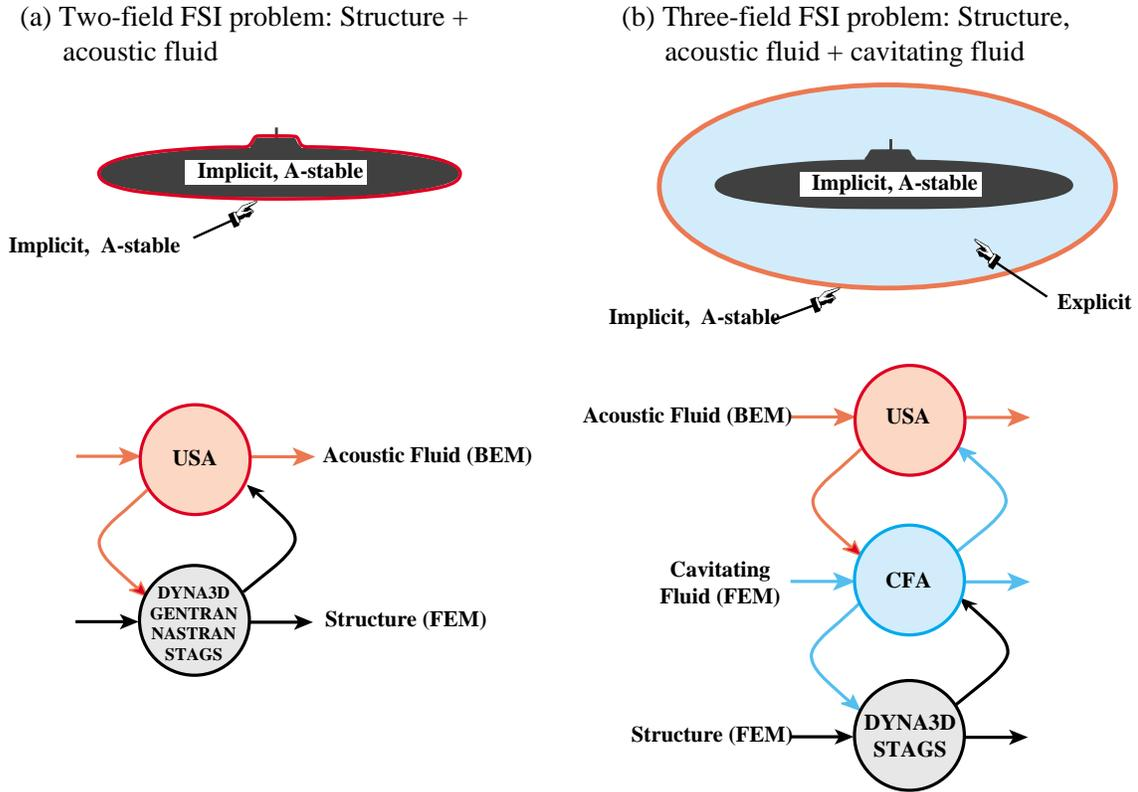
Figure 11. Implementation of partitioned analysis treatment of underwater shock analysis: (a) as two-field problem coupling acoustic fluid and submerged structure models, (b) as three-field problem coupling acoustic fluid, cavitating fluid and submerged structure models.
