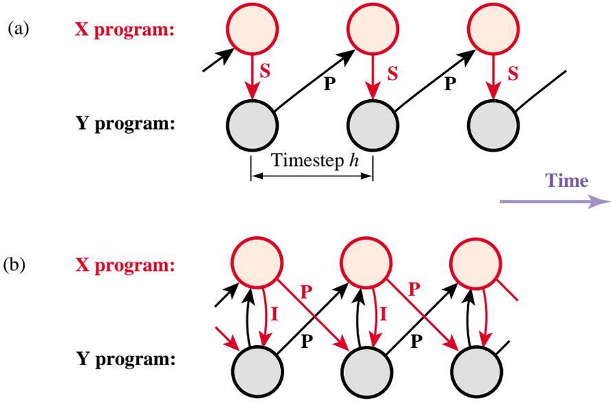
Figure 7. Interfield time stepping diagrams: (a) sequential staggered solution of example problem, (b) naive modification for parallel processing.
