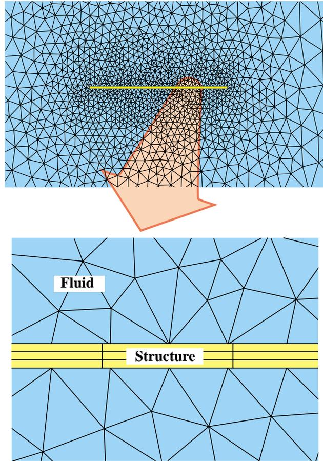
Figure 2. Differential partitioning was originally developed for fluid-structure interaction problems, in which nonmatched meshes occur naturally.
