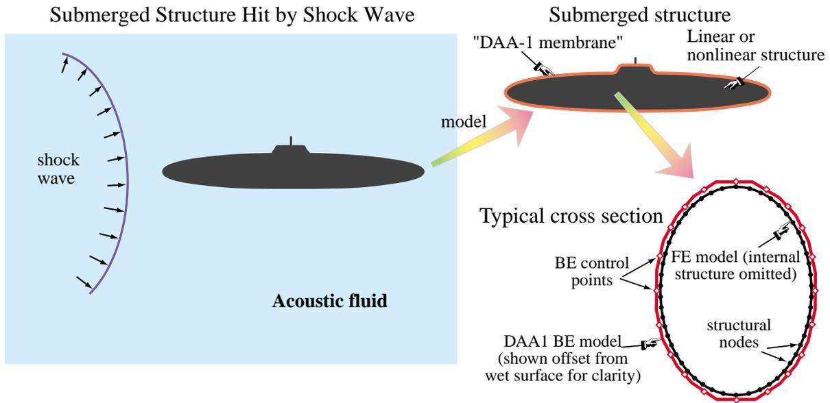
Figure 9. Submerged structure hit by shock wave: (a) physics of the coupled system, (b) acoustic fluid modeled as “DAA<sub>1</sub> membrane” (c) typical cross-section of coupled FEM-BEM discretization on the wet surface with the interior structure omitted. In (b) and (c) the BEM fluid model is shown offset from the structure for clarity.
