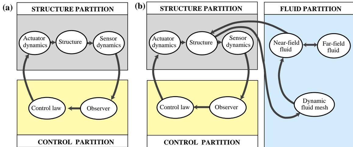
Figure 14. Active control of dry and wet structures as (a) two-field, (b) three-field coupled systems.
