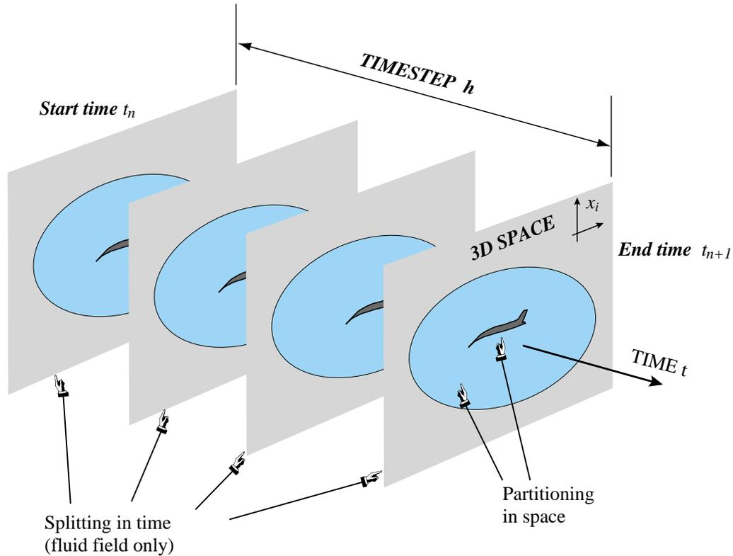
Figure 1. Decomposition of an aeroelastic FSI coupled system: *partitioning* in space and *splitting* in time. 3D space is shown as “flat” for visualization convenience. Spatial discretization (omitted for clarity) may predate or follow partitioning. Splitting (here for fluid only) is repeated over each time step and obeys time discretization constraints.
