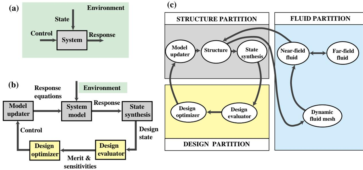
Figure 16. Computer driven design and optimization of a wet structure as component of a coupled system: (a) abstract interpretation as optimal control problem, (b) practical computer implementation, (c) partitioned analysis diagram.
