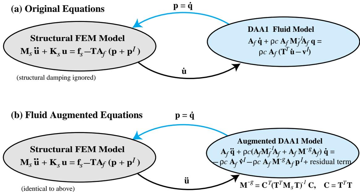
Figure 12. Reformulation of two-field semidiscrete FSI equations: (a) original (after some DAA<sub>1</sub> rearrangements), (b) upon augmentation of fluid model by structural terms. Augmentation permitted A-stability to be retained in staggered solution.
